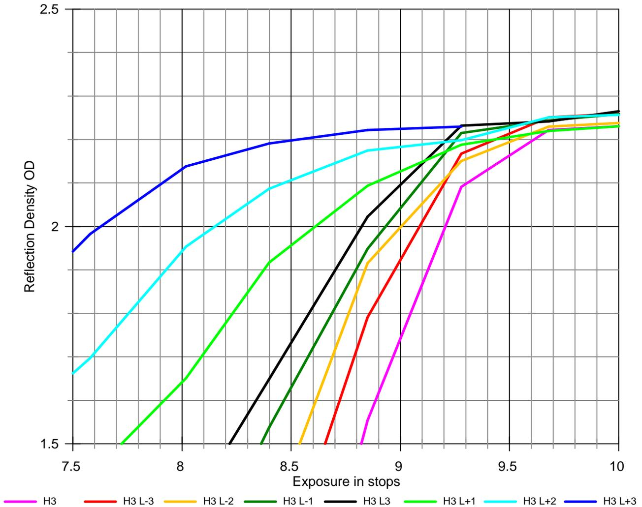
In the expanded view, above, note that the normal (black H3 L3) through high contrast (red H3 L-3) curves all cross the 2.1 density line within 0.2 stops of each other. The low contrast exposure has little effect on the black-point exposure for high contrast prints.
