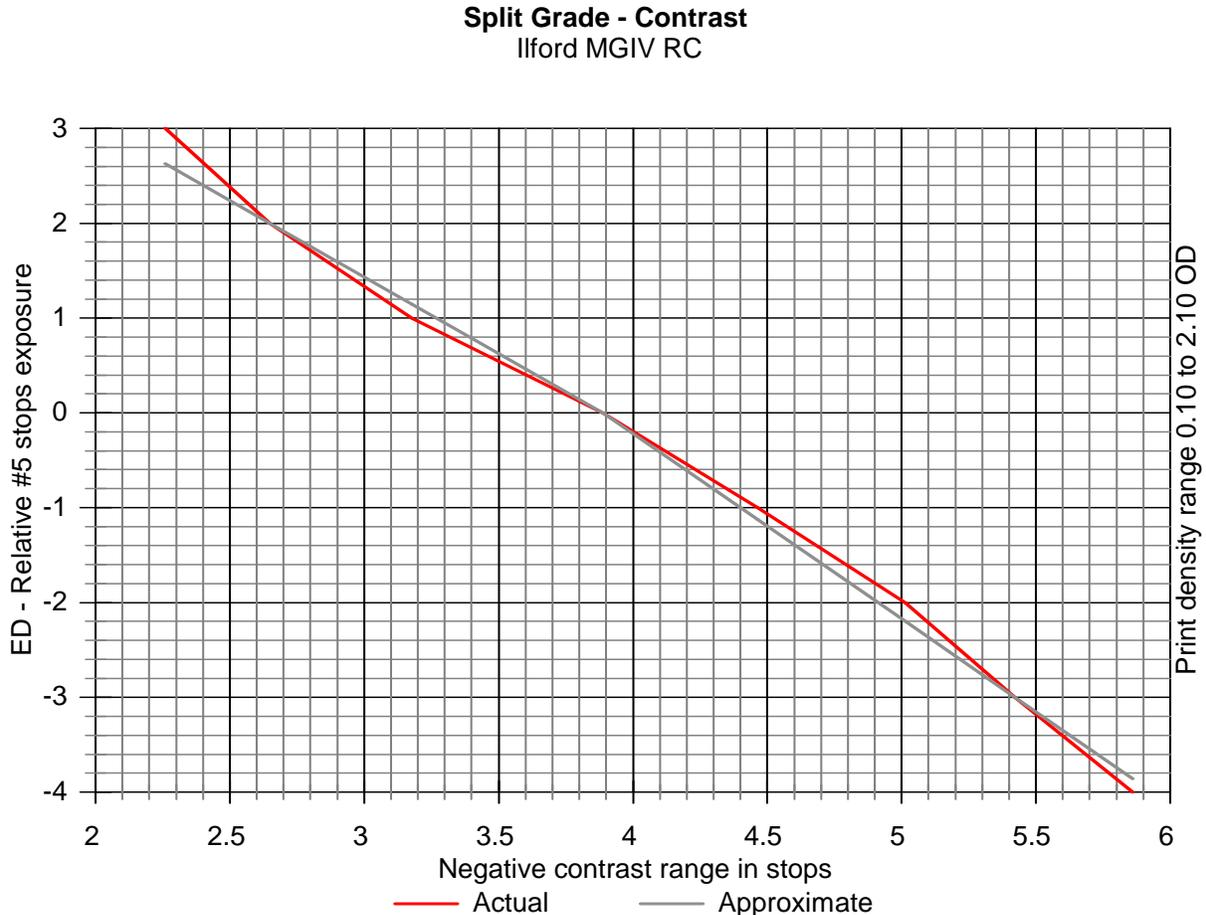
Note the approximate curve is derived from the quick paper characterization method given later in this application note.
