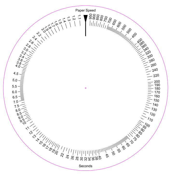
Cut volvelle along the magenta lines. Attach the back to foam core or cardboard and pin the cursor and inner wheel at the center.
