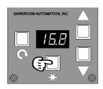
Start the exposure by tapping the expose key. The enlarger will turn on and the safelight off, the display will count down the remaining seconds.
