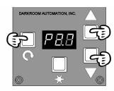
After making the base burn as shown above, press the mode key to advance to progressive burning - 'p' will show in the display. If there are no progressive burns then advance to base exposure, otherwise set the number of stops to burn.
