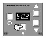
Make an exposure with the strip covered. At the end of the exposure the timer will flash the total exposure given to the last strip.
