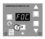
You can focus at any time by holding the expose key down for one second. Turn the enlarger off by tapping the expose key again.
