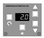
The timer is ready to make the base exposure when there is a blank character in the left position.
